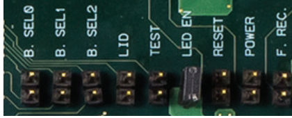
Figure 49: Jumpers for Boot Select
