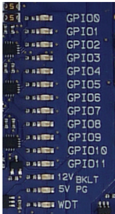
Figure 12: GPIO and Backlight LEDs, see board position 19
